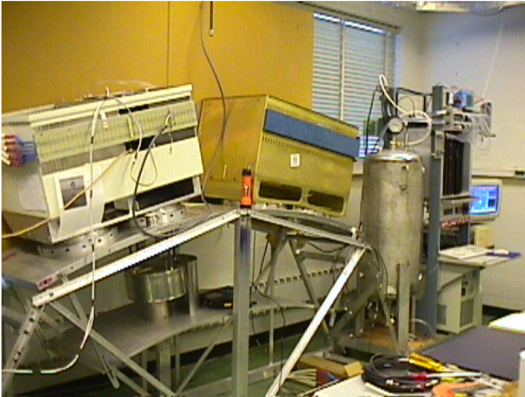
Figure 16: Laboratory mockup of two crates. A water cooling system is shown at the back. The curved surface simulates the ends of the cryostat. One 'open' feed through is also seen.
