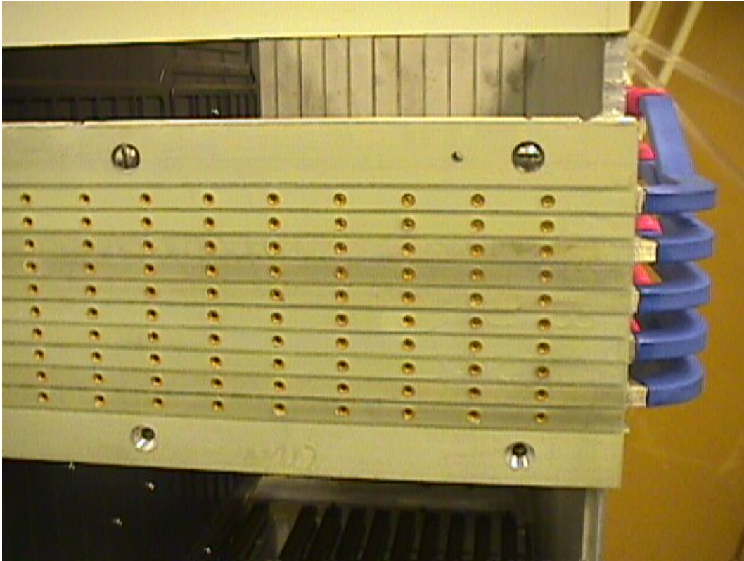
Figure 9: Power Bus prototype. The bus bar is built starting by gluing 10 copper lines ( 1/4 \times 0.400 ) and two aluminum mounting bars. After the curing time of the epoxy, the bus bar is mounted on a NC machine for precision drilling. Inserts are then press fitted and bus bars terminated.
