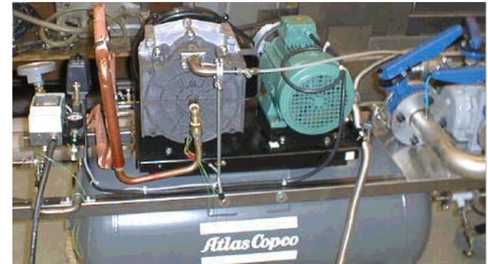
Performance test with modified Scroll compressor
