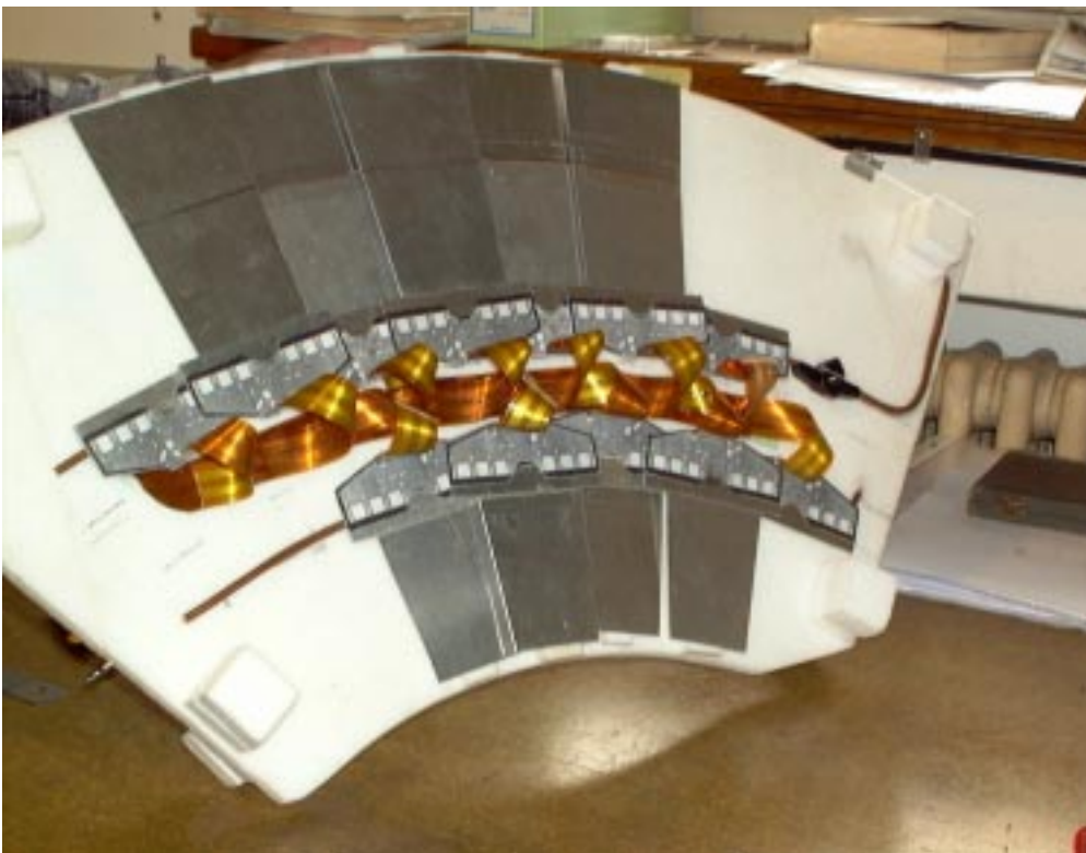
Figure 18: Disk sector mock-up including mechanical modules, cooling pipes and cables.
