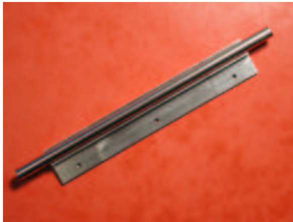
Fig. 3. Aluminum cooling block prototype (“split block design”).
