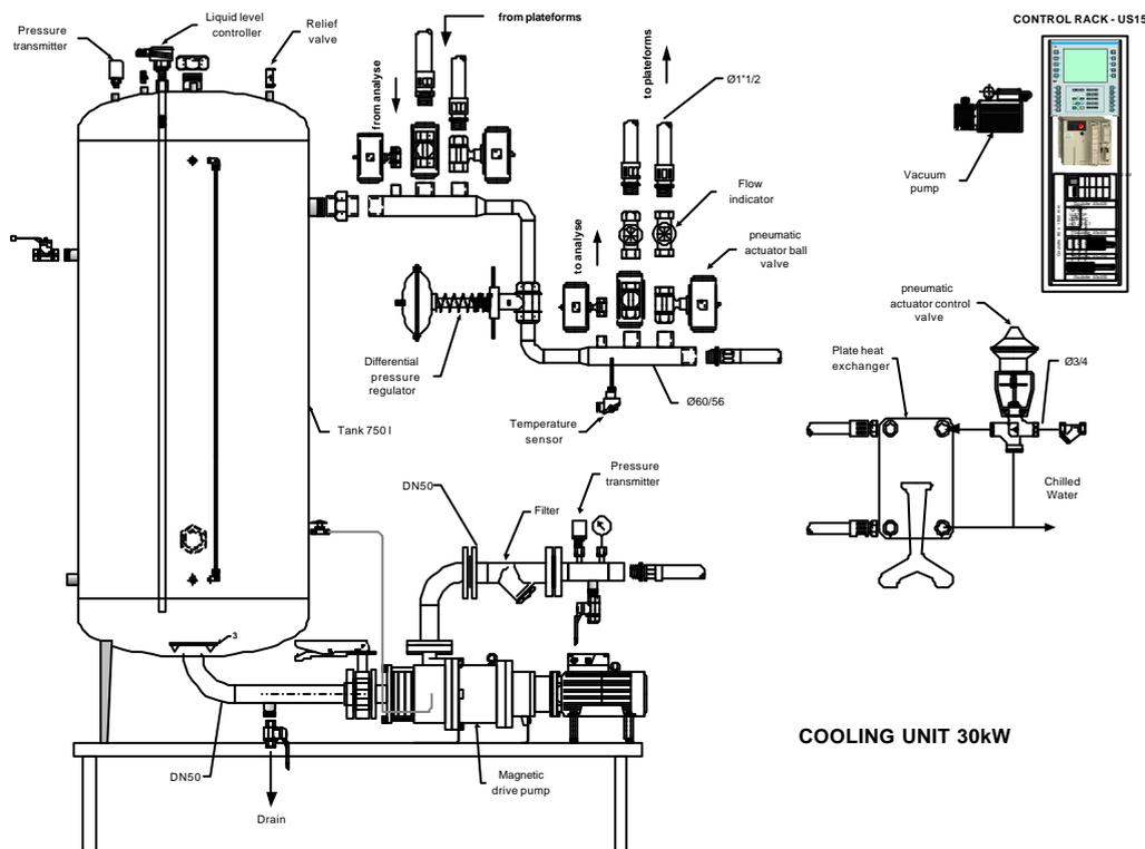
Figure 6: The cooling unit with its main components
