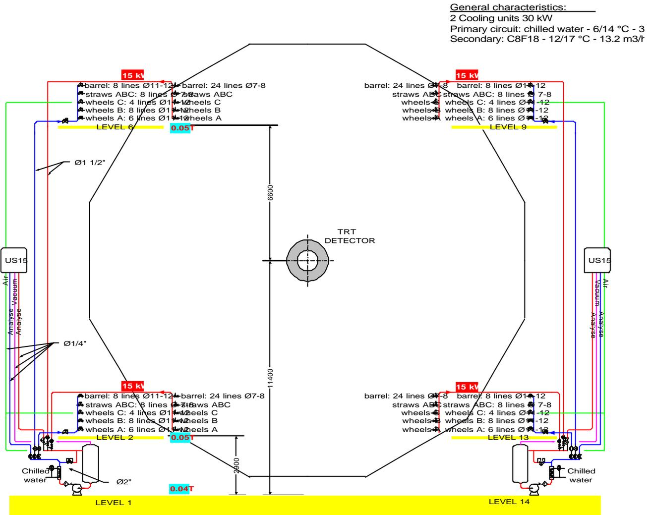
Figure 7: Layout of the TRT cooling system in ATLAS experimental cavern
