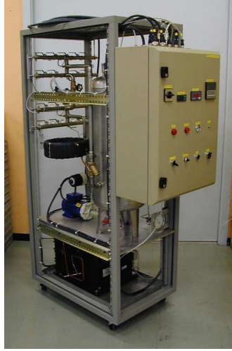
Figure 4.1: Cooling station used for the Cs calibration of the Tilecal modules. The unit is independent and movable.
