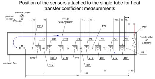
HT (1,2) - coil heater-thermometers
